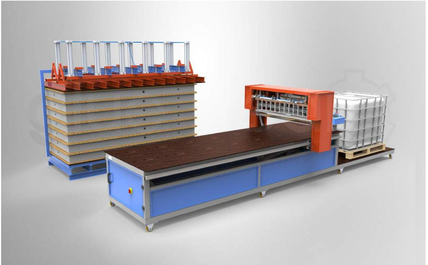
**Adhesive extruder SPL-9** is designed for automatic applying 1-C PUR adhesives on the upper surface of the bonding substrates.
