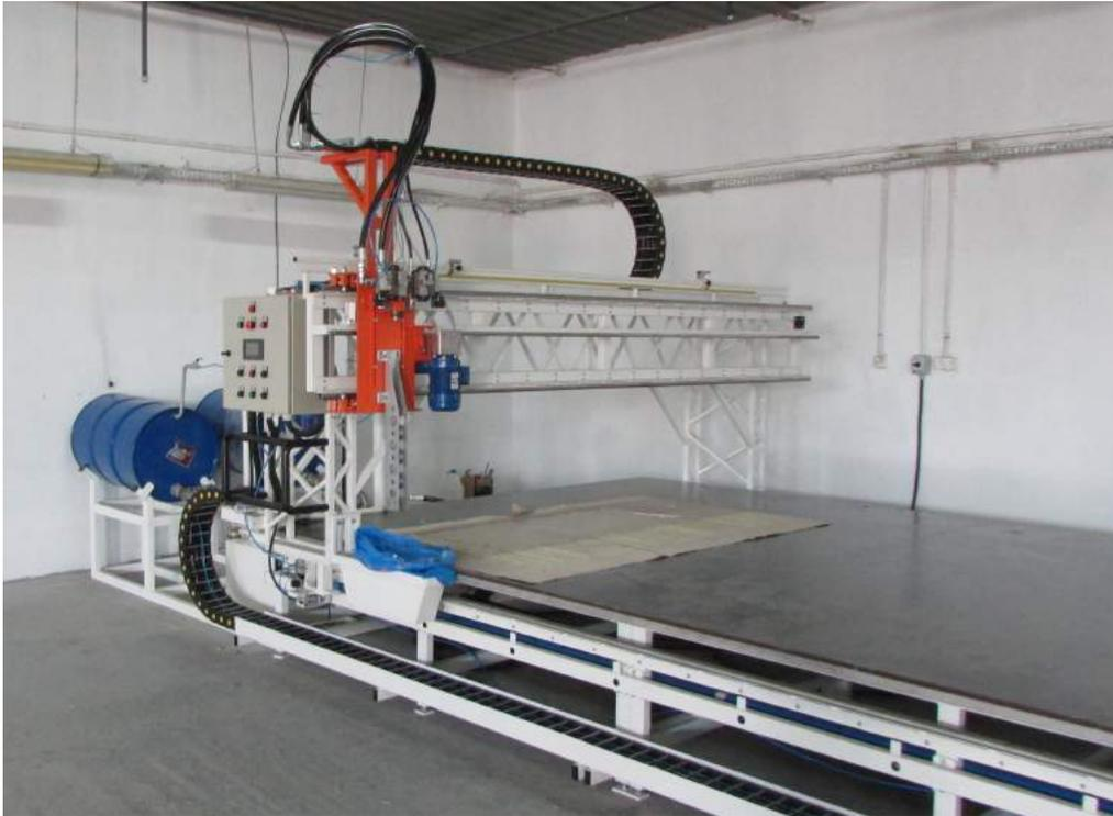
Adhesive applying machine for large panels **KAM VAN-Portal Mini** is designed for precisely metered application of two component adhesives with semi-motorized applicator along the working table width.
