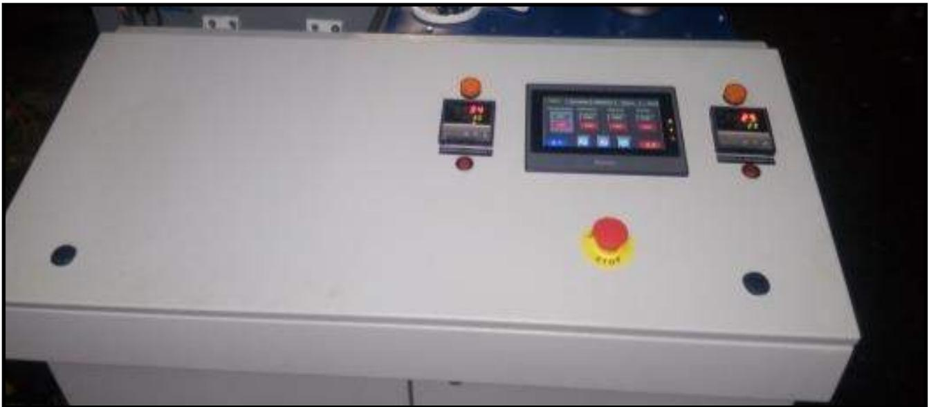
The interface language of the control panel can be installed according to the customer's requirements. The front part of the electrical cabinet also includes thermostats of the components, for temperature control and thermo stabilization control, light indication of the sensors of the minimum level of components, emergency stop button.
