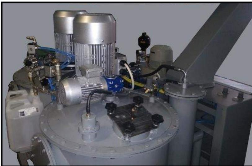
The axial-piston pumps are used for dosing the components A and B. The dosing pumps are electrically operated, their speed is regulated by a frequency converter, which receives commands from the control panel. The accuracy of the dosing and the mixing ratio is controlled by flowmeters. Dosing pumps are located in the tanks of the components.
